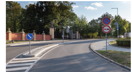
Figure 10: Anomalous and irrelevant use of overtaking signs in built-up area
