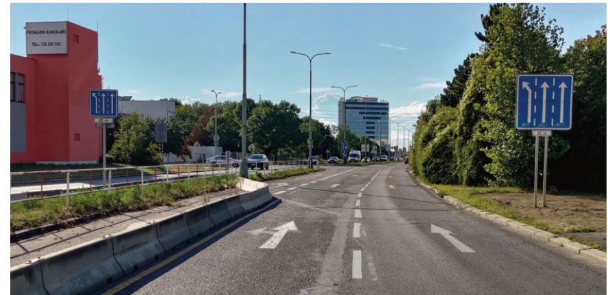
Figure 2: Comparison of smaller and standard lane sign sizes on arterial road.
