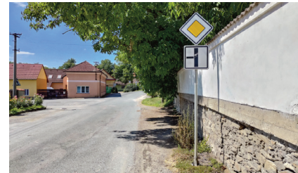
Figure 11: Redundant additional plates showing standard intersection diagram.
